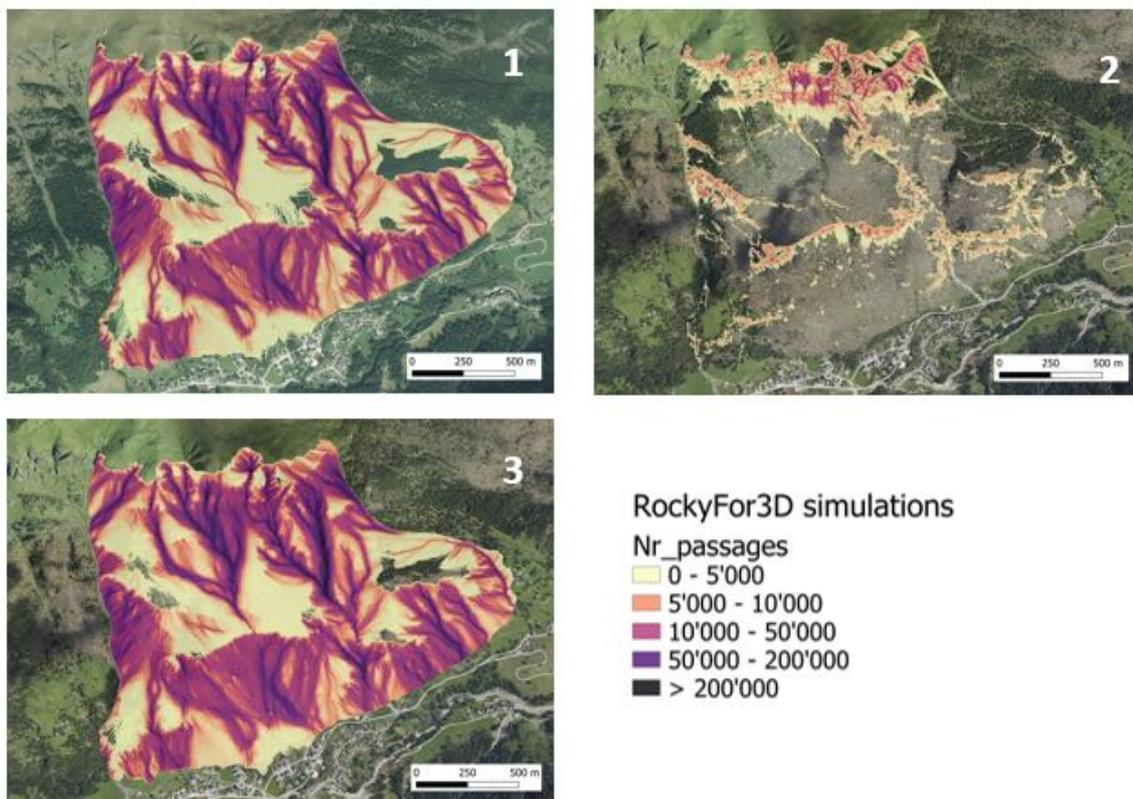
Figure 16. Simulations outputs for BoscoVerde, fraction of Rocca Pietore municipality. Simulations scenarios are 1) before the storm, 2) after the storm, 3) after salvage logging
