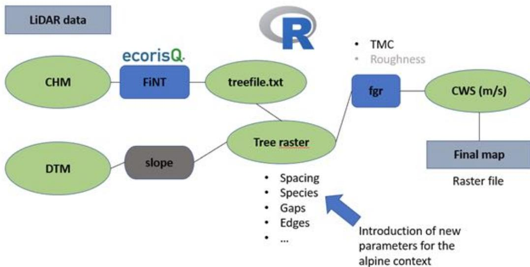
Figure 11. Workflow for wind susceptibility mapping that was applied. It is possible to observe where it was possible to use the new parameters of fgr model, it is also highlighted that fgr model was run with the TMC method.
