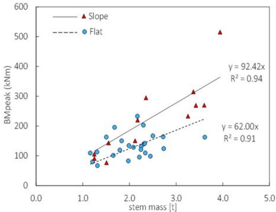
Figure 9. Stem mass (t) against Bending Moment (kNm), blue dots are referring to trees growing in flat conditions, red dots are referring to trees growing in steep terrain (figure from Marchi et. al, sub)
