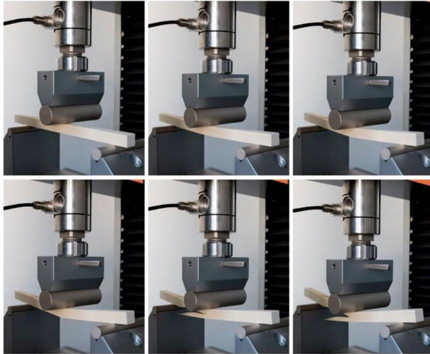
Figure 10. Procedure for the evaluation of MOE and MOR of wood samples. Samples were coming from the tested trees in Valmenera. (ph. Matteo de Mayda)
