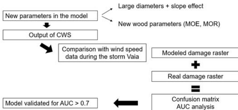
Figure 2. Validation flow-chart for fgr, based on a work by Hale et al (2015)
