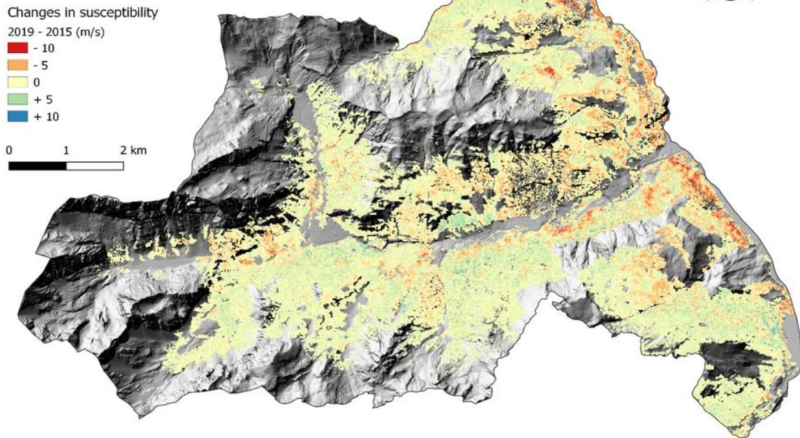
Figure 14. Changes in wind susceptibility due to the storm Vaia, the map was obtained subtracting 2015 from 2019 data
