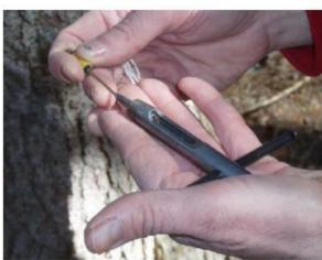
using the "extratcing needle" push lightly the microcore on the top ...
